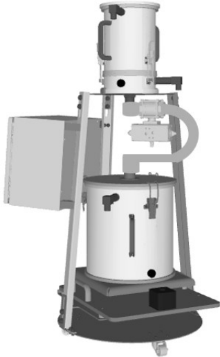
Scheme of the laboratory test rig for dewatering measurements (© Photo: Wood K plus)
