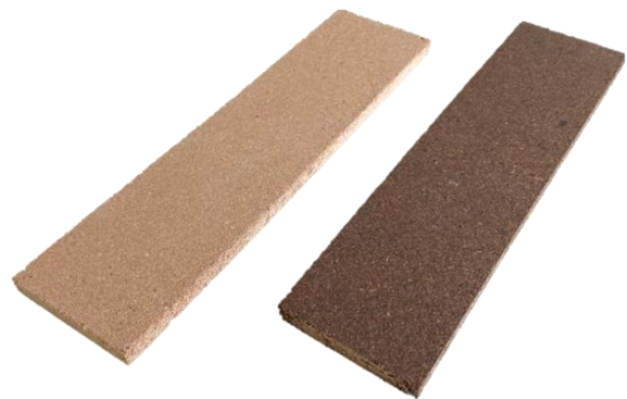
100% bio-based panel materials based on 90% beech wood dust (left) or 90% oak wood dust (right) and 10% polyhydroxyalkanoate (© Photo: Wood K plus)
