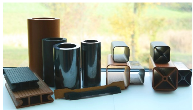
Various geometries of WPC green bodies, porous carbons and SiC ceramics (© Photo: Wood K plus)
