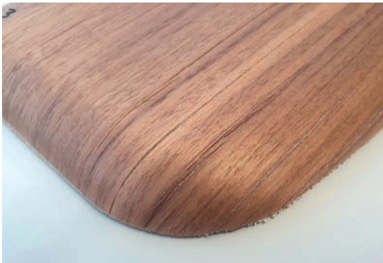
3-dimensional umgeformtes Organoblech mit Naturfasergewebe (links) und Walnuss-Echtholz furnier (rechts) 3-dimensionally formed organo sheet with natural fiber fabric (left) and walnut real wood veneer (right)
