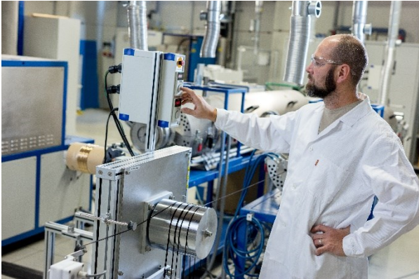
© UAR, Photo by: Hartwig Zögl: Wood K plus employees at the tube furnace during the production of carbon fibers from cellulose
