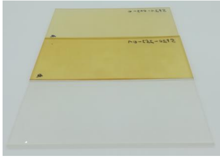
Figure 3: Considerable yellowing after artificial weathering in xenon test chamber (© Wood K plus)
