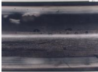
Figure 7: Air bubbles at the surface of the fibre due to insufficient pre-drying (© Wood K plus, Chethan Savandaiah)
