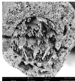
Figure 6: SEM picture of a composite extrudate with short-CF-reinforced matrix produced with 3D printer Composer A4 (© Wood K plus, Chethan Savandaiah)
