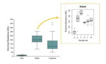
First results of the resistance measurement on spruce wood provide information about the statistical distribution of the electrical wood properties between different samples. © University of Natural Resources and Life Sciences, Vienna
